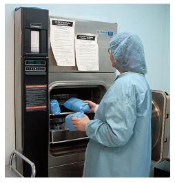
FIGURE 12-11 An autoclave.
